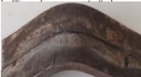
Gambar 6. Hasil uji bending 100A
